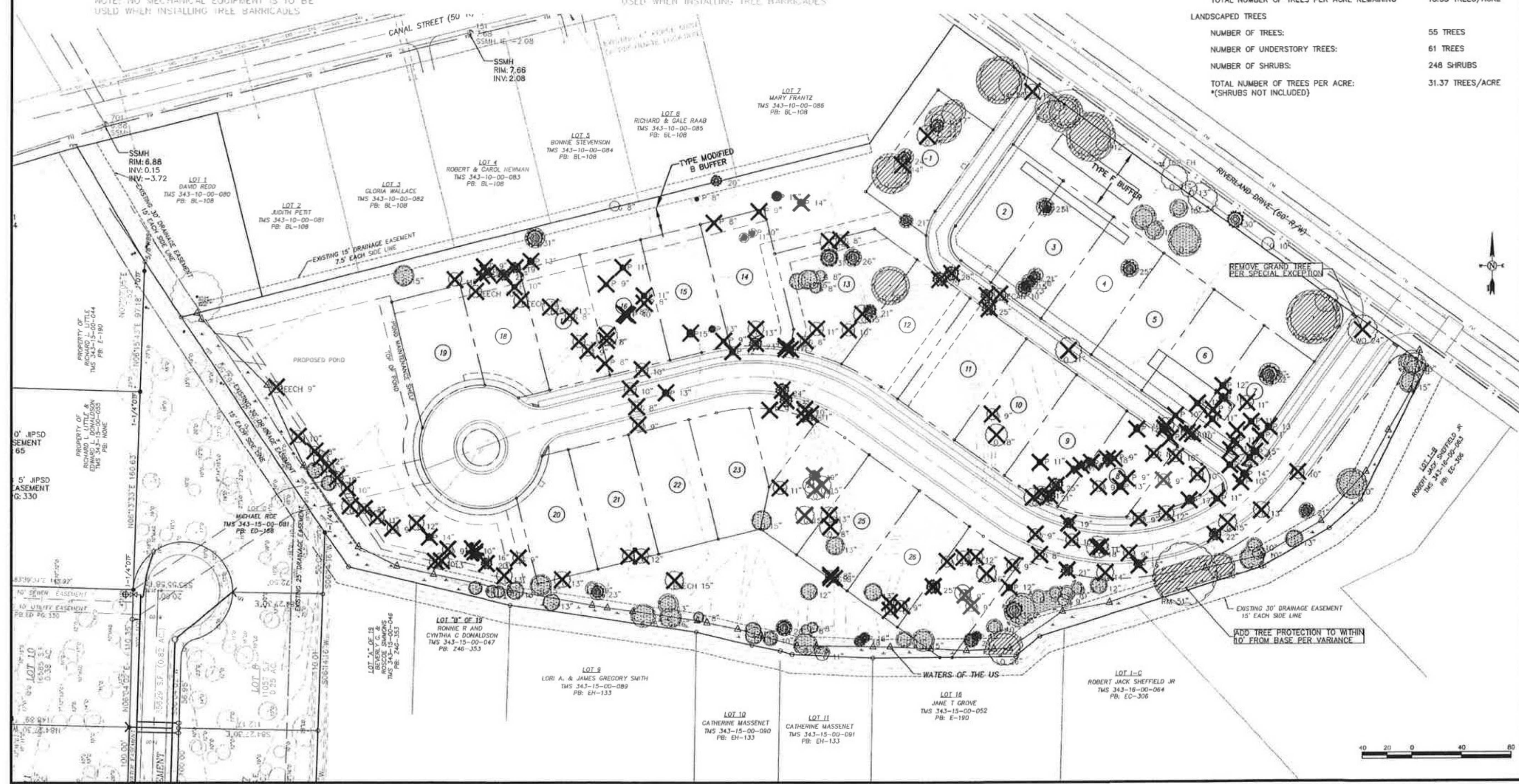
TREE PROTECTION - SAFETY FENCING NOTE: NO MECHANICAL EQUIPMENT IS TO BE USED WHEN INSTALLING TREE BARRICADES
